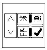
The Driver Information Center (DIC) has different displays which can be accessed by pressing the DIC buttons located on the instrument panel, to the left of the steering wheel. **Trip/Fuel:** Press this button to scroll through the trip and fuel displays. See "Trip/Fuel Display Menu Items" following for more information on these displays.
